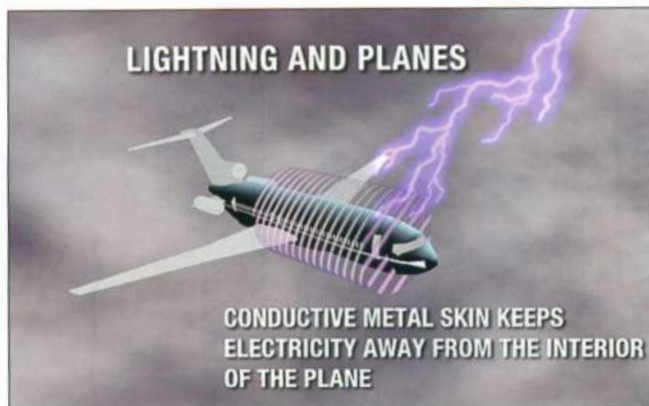
Acting as a "Faraday Cage," metal skins and frames help shield interior electronics and passengers from lightning. Nonmetallic skins often contain a layer of conductive material for the same purpose.
