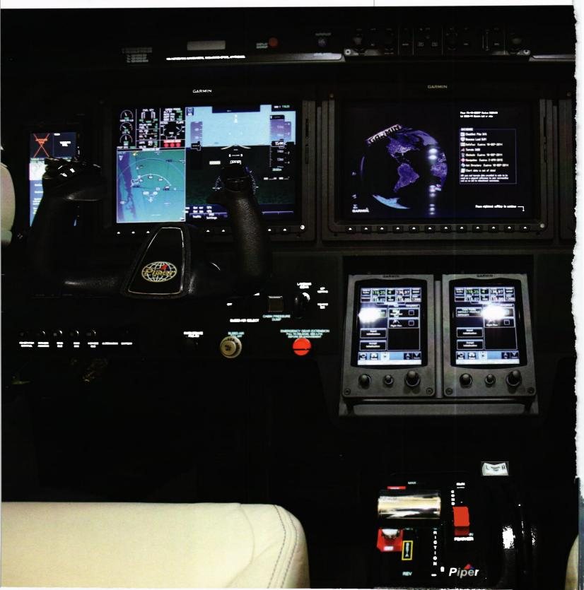
this system displays the more accurate of • GMA-350 Audio Panel: With features such as 3D Audio for split feeds and Blue Select entertainment distribution for fine tuning XM music and phone interface. • EFD-1000 Aspen Standby System: Replaces the wet compass and provides a very capable and reliable back-up system. MAN SHALLS
